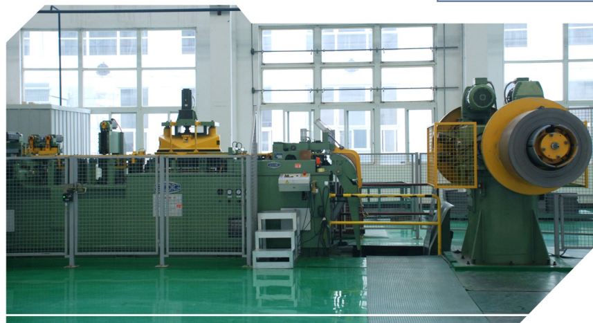
德国TBAMEEL800 × 5000乔格变压器铁心片横剪生产线 Germany TBAMEEL800 × 5000 lamination cut-to-length line from George company in Germany
