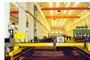
HQCS5000 x 14000FP(E)数控火焰等离子切割机 Digital-controlled plasma flame cutting machine
